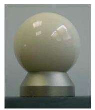
The ceramic probing spheres of  $\emptyset$  30 mm is standard (other diameters are possible) are fixed mechanically in a tapered seating such that adhesive cannot influence the sphere position in a negative way.
